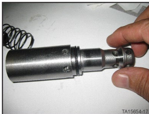
Anti-Void Spool Assembly removal
