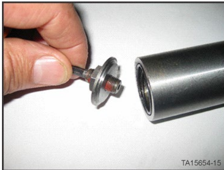
Relief Valve Adjustment Screw installation
