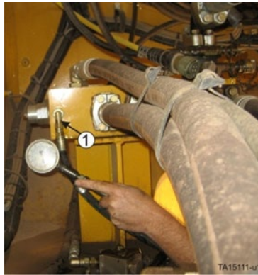
1) Outlet of the auxiliary steering pump output hose
