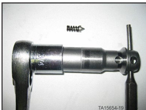
Valve Seat removal
