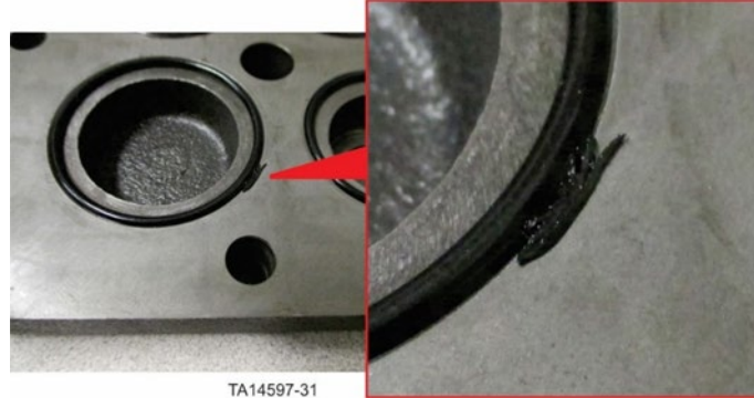
Example of a damaged O-ring
