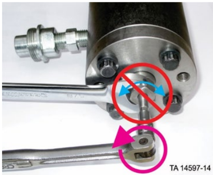
Hold jam nut, turn adjustment shaft counter clockwise
