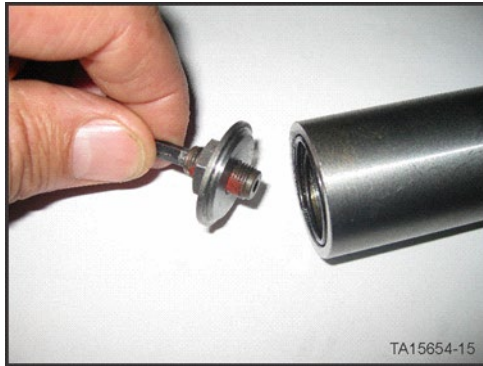
Loosening of the adjustment screw jam nut (original non-modified adjustment screw shown)
