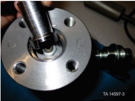
Align the flats to the jam nut
