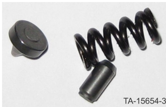
Example of broken cone
