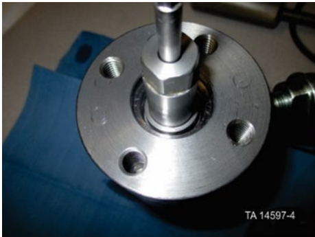
Place the tool on the jam nut
