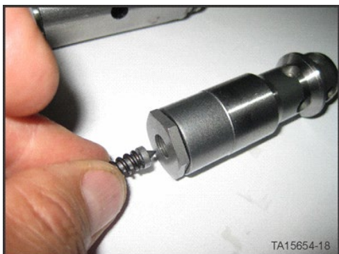
Relief Valve Cone and Spring removal
