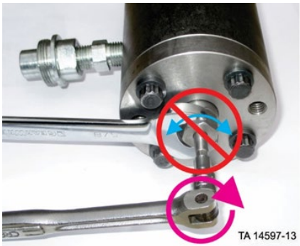
Hold jam nut, turn adjustment shaft clockwise
