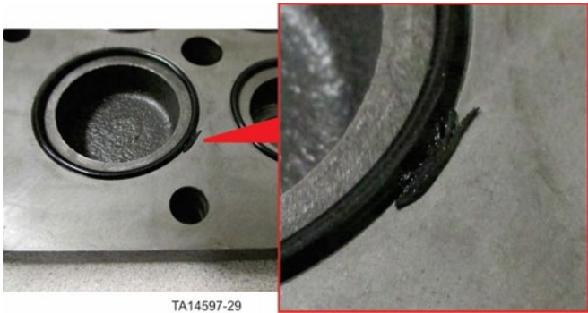
Seal Inspection (Damaged seal shown for example purposes)
